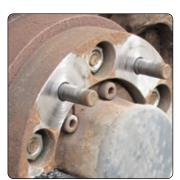
Special grinder used to clean the wheel rim contact surface, designed for vehicles with stud bolts. Corrosion is quickly and easily removed. For use with Impact.
